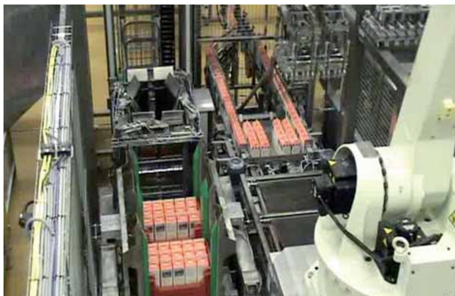
View inside the robot cells which load the filled cartons into roll containers or crates
