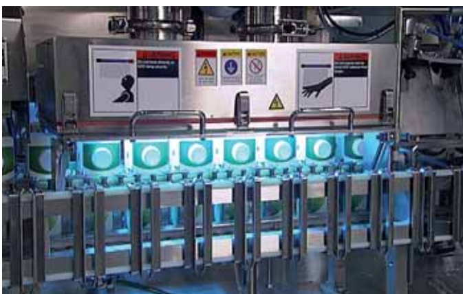
UV light decontamination of cartons
