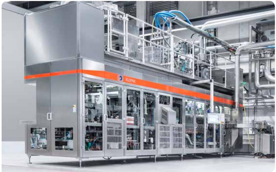
Elopak's newest filling machine E-PS120A for Pure-Pak® aseptic cartons.
